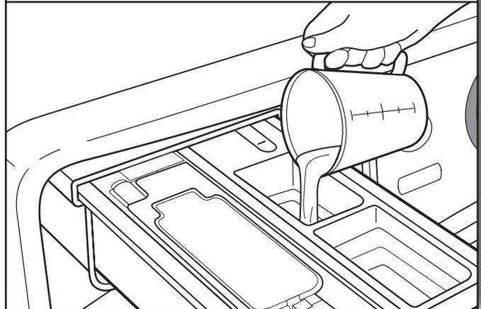
Add liquid chlorine bleach to the bleach compartment. Do not overfill, dilute, or use more than ⅔ cup (165 mL). Do not use color-safe bleach or Oxi in the same cycle with liquid chlorine bleach.
