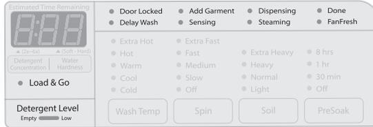
The Cycle Status Lights show the progress of a cycle. At each stage of the process, you may notice sounds or pauses that are different from traditional washers.
