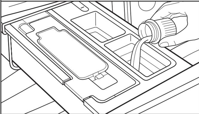
Pour a measured amount of liquid fabric softener into liquid fabric softener compartment. Always follow manufacturer’s directions for correct amount of fabric softener based on your load size.
