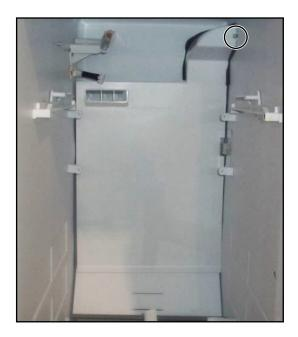
2. Once freezer cover gets off then push on the tabs in the air supply area and this will push the damper out.
