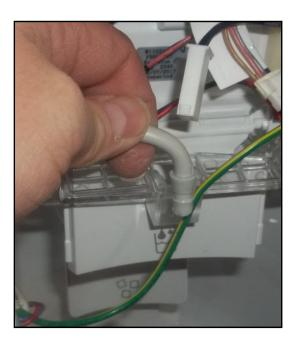
**6.** To remove ice door, remove water line for the holder. Remove the upper screws then pry tabs.
