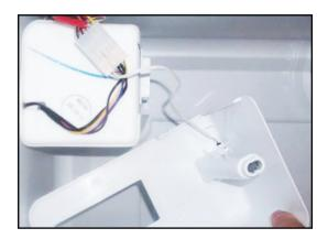
5. The damper will come out. The damper has both RC and FC thermistor on the harness.
