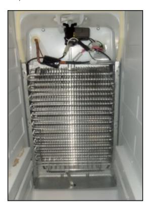
**3.** Below picture shows freezer components. Defrost thermistor goes on the cap tube side.
