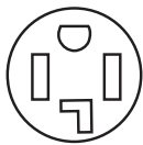
4-wire receptacle (14-30R)
