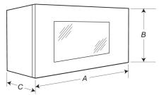
A. 29<sup>7</sup>/<sub>8</sub>" (76.1 cm) B. 17<sup>7</sup>/<sub>8</sub>" (45.4 cm) C. 12<sup>1</sup>/<sub>8</sub>" (31.3 cm)
